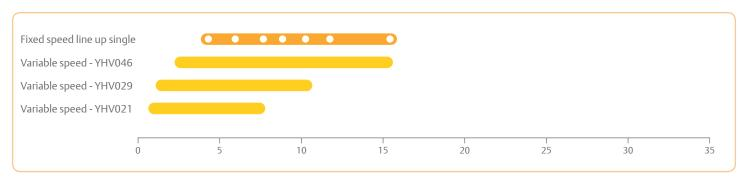
Heating conditions in kW: evaporating -7°C, condensing 50°C, superheat 10K, subcooling 4K
