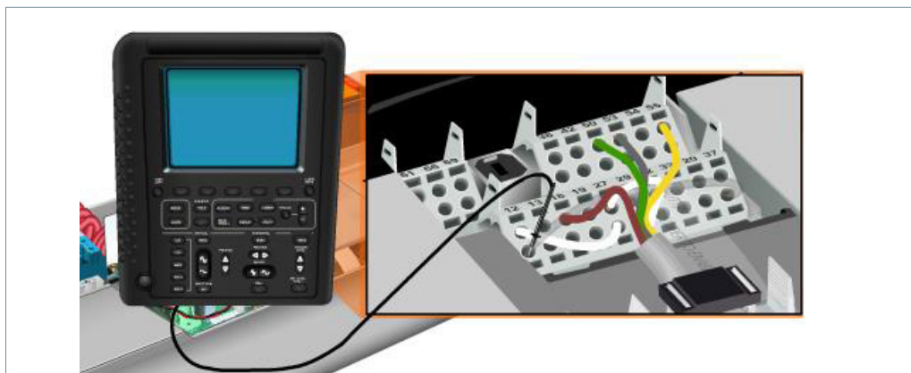
Figure 10: checking control signal in the control card
