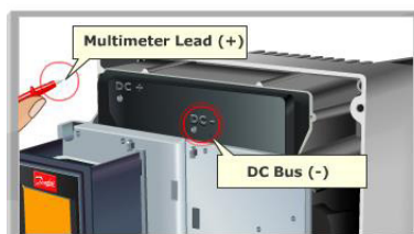
Figure 15: The multimeter should show diode open
