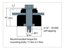
act ıg sleeve is established. The required bolt size for the LLZ013-034 compressors is M8\*45mm. This bolt must be tightened to a torque of 11 Nm.
