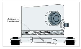
It is recommended that the heater be turned on for a minimum of 12 hours prior to starting the compressor.
