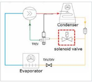
Liquid injection system configuration
