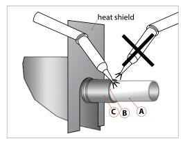
R Before eventual un-brazing of the compressor or any system component, the refrigerant charge must be removed.
