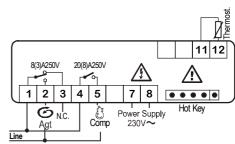
12Vac/dc supply: connect to the terminals 7 and 8. 24Vac/dc supply: connect to the terminals 7 and 8. 120Vac supply: connect to the terminals 7 and 8.
