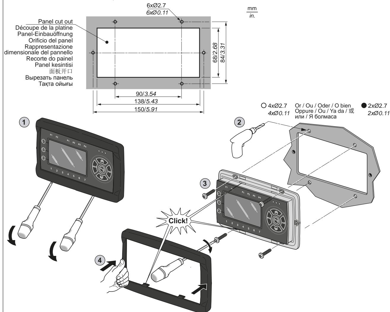
Wall mounting / Montage mural / Wandmontage / Montaje en pared / Montaggio a parete / Montagem na parede / Duvara montaj / 墙壁安装
