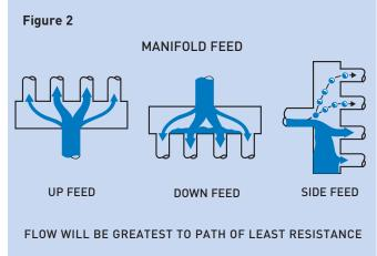
To achieve proper distribution, the liquid portion of the two-phase flow must be divided equally to each evaporator coil circuit. The solution: [1] mix the liquid and vapor portions of the refrigerant flow; and [2] maintain a homogeneous two-phase mixture until equal portions of the flow are divided into each evaporator circuit.
