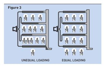
Optimum distributor performance is obtained when the distributor is mounted directly to the TEV outlet. If the distributor cannot be mounted directly to the valve outlet, it can be connected by a piece of **straight** tubing or pipe. The tubing or pipe should not exceed **two** feet, and it should be sized to maintain high refrigerant velocities. Elbows located between the TEV and distributor hinder proper distribution, and are **not** recommended.
