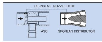
As with side connection type Sporlan distributors, the ASC allows hot gas or liquid refrigerant in the reverse cycle to bypass the nozzle. In addition, the two-phase refrigerant flowing from the TEV passes through the nozzle, and a nozzle tube extension, which terminates at the distributor's
