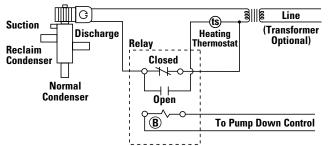
When the pump down control is energized, relay coil (B) is energized. This allows the heating (s) to control the 3-Way Heat Reclaim Valve operation.
