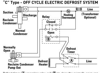
Defrost timer (A) energizes relay coil (B) to close the normally open contacts. This bypasses the (t) when defrosting to close the pump out solenoid and shut off the valve's pump out to suction.
