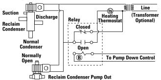
When the pump down control is energized, relay coil (B) is energized. This allows the heating (s) to control the 3-Way Heat Reclaim Valve operation.
