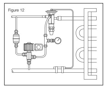
By successively opening and closing the circuit to the Pilot Control only, with the refrigeration system and circulating fans or pumps in operation, variations approximating condensing pressure and suction pressure should be observed on this gauge.
