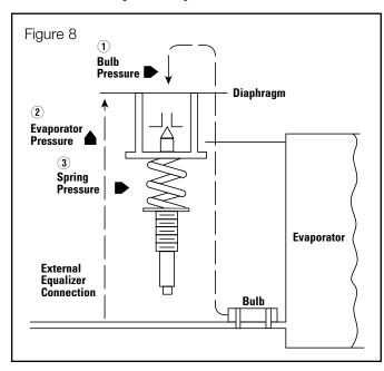
superheat at the outlet of the evaporator. However, when an abnormal pressure is introduced which upsets the equilibrium, another effect may be accomplished. The principle upon which the 180 Solenoid Pilot Control influences the expansion valve action is by the creation of a pressure under the valve diaphragm, which is higher than the bulb pressure. This is how it is accomplished.
