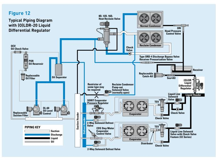
A normally open OLDR version or an LDR version (differential mode when the coil is de-energized) must be determined if a liquid differential pressure regulating valve is desired.
