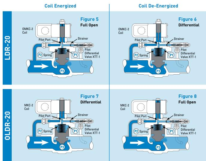
the main piston. These valves are available in two port sizes, the (O)LDR-16 (1") and the (O)LDR-20 (1-5/16"). Inlet pressure enters the pilot assembly through a passageway in the valve body on the (O)LDR-16, and through an external tube connected to the inlet fitting on the (O)LDR-20. The outlet on the pilot differential is through an internal passage in the valve body on the (O)LDR-16, and on the (O)LDR-20, the valve is connected to the outlet fitting with an external tube.
