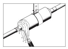
All sealed model suction line filters and filterdriers have copper fittings. It is not necessary to clean the fittings prior to brazing.
