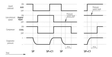
The unit alerts users via a message on the screen, by activating a relay $^*$  or both, when the programmed parameter criteria are met.
