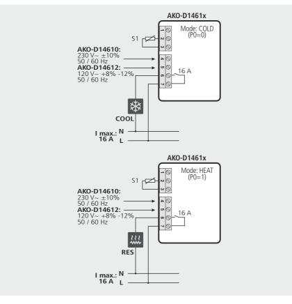
5.3.-2-relay controller (Control + Alarm)
