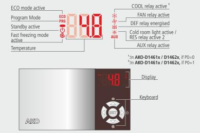
Flashing lights indicate that the function in question should be activated by temperature, but is not due to a conflicting timing or protection parameter.
