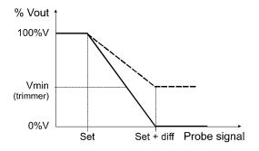
If the input signal is lower than the Set, the output signal is 230 Volt (fans are running at the maximum speed). When the signal increases and enters the range between the Set and Set+Diff the output signal follows the temperature variation. Above the Set+diff value the output signal is always 0 Volt (if no Vmin has been set).
